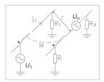
Interference voltage  $(U_n)$  is proportional to the frequency (f) and current  $(I_1)$  of the interfering conductor and to the mutual inductance of the circuits  $(M_{12})$ . Mutual inductance is proportional to the area of the loop perpendicular to the magnetic field lines (A cos  $\theta$ ) devided by the distance between the conductors (r):
