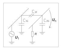
Interference voltage ( $U_n$ ) is proportional to frequency (f), voltage level of the interfering conductor ( $U_1$ ) and stray capacitance between the conductors ( $C_{12}$ ):
