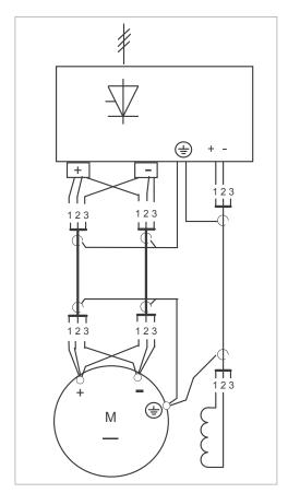
The excitation cable is a heavy source of interference because of the abrupt commutation. Therefore, always use shielded excitation cables.
