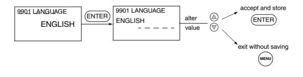
Note! In the parameter value set mode the cursor blinks, when the parameter value is altered.
