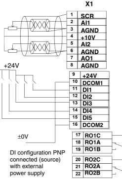
Figure 5 ACS 400V I/O connection.
