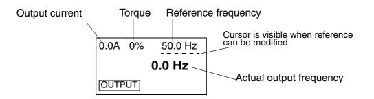
The frequency reference can be modified using UP/DOWN buttons when it is underlined. Pressing UP or DOWN buttons changes the reference immediately.
