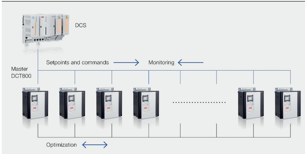
Communication architecture of the DCT880 (4)
