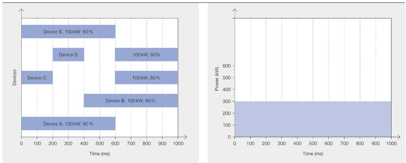
During the cycle some consumers can be switched on and off twice (9a) Splitting is the only way to reach a perfect solution (8b)
