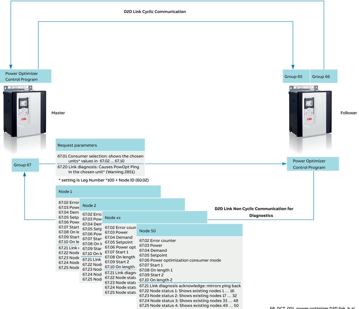
Power Optimizer non-cyclic diagnostic communication schematic
