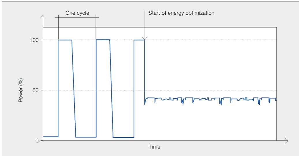
Energy consumption (relative to the sum of the power of all heaters) of an installation with 14 consumers without (left half of graph (5a)) and with (right half (5b)) power optimization (5)
