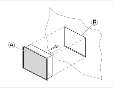
Assemble the four mounting brackets and fix these to the control panel in the mounting plate as shown here (tightening torque: 0.75 Nm).
