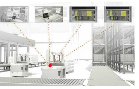
A modern distribution center comprises several independent systems including conveyor and lift systems, robotic sorting and palletizing processes, together with autonomous guided vehicles, or AGVs, and automated stacker cranes that lift pallets to and from the high bay storage systems.
