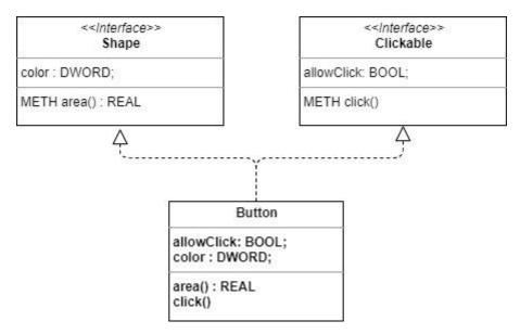
Also a combination of Implementing and Extending is possible. Similar pictures shown above a Button could also implement Clickable and extend Rectangle. Then the method area is predefined in Rectangle.
