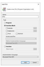
The Function Block is the main Object for OOP and can be treated as class which can have several instances. The new possibilities in V3 which extend the functionality in V2 are described in chapter 3.1.
