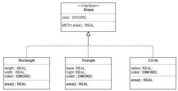
In contrast to the extending of function blocks one function block can implement multiple interfaces. For example, the function block Button can implement the interface Clickable and Shape.
