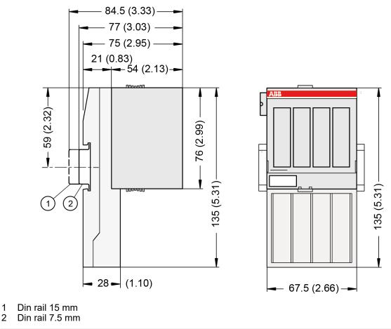
The dimensions are in mm and in brackets in inch.
