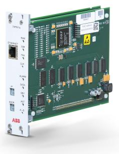
The 70PR07a may be employed for a variety of control and automation duties. It is operated individually or in conjunction with other processing module in a local bus station. The module operates with the bus traffic director 70BV05 and controls I/O based on stored user programs (AWL), communications with the P13 local bus. The 70PR07 mounts into a local bus sub rack and receives communications and power from the local bus back plane.
