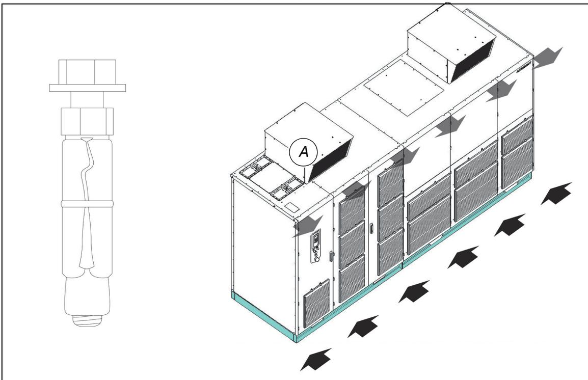
*Fixing the base to the floor*
