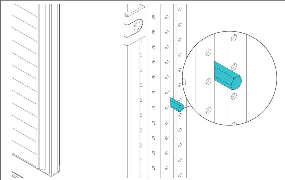
Floor fixings are not supplied. M16 anchor bolts as illustrated in figure below, or screws, nuts and washers of size M16 are recommended (diameter of holes in base frame: 18 mm). It is prohibited to solder the drive to the foundation.
