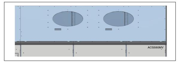
2. Use the supplied screws to fasten the fan units to the cabinet roof.
