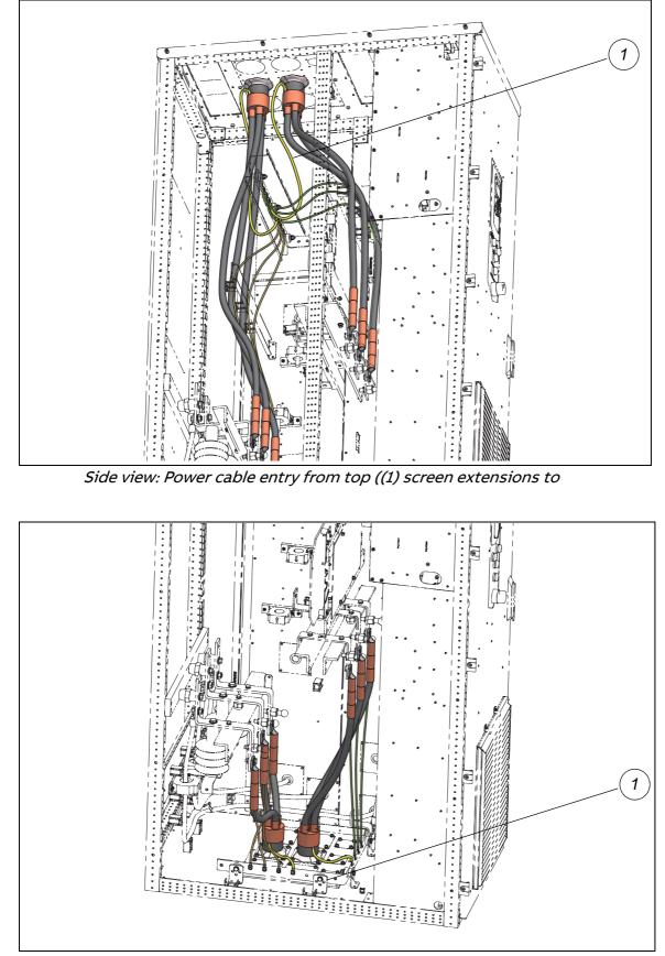
Side view: Power cable entry from bottom ((1) screen extensions to
