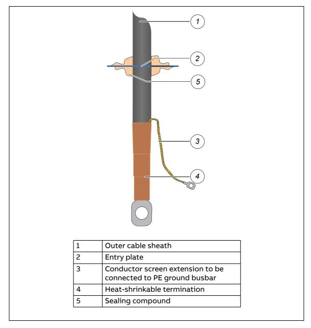
Connect the cables to their corresponding busbars. Use cable lugs suitable for M12 bolts. The required tightening torque is 40 Nm.
