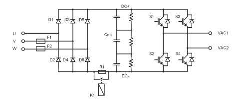
Figure 6: R1-R6 power modules main circuit diagram
