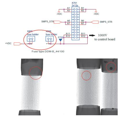
Fuse on HCB of power module open and cause control board cannot work.
