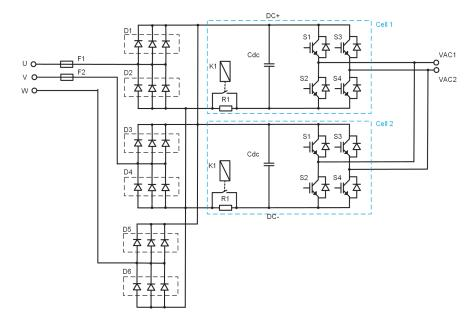
Figure 8: R8 power module main circuit diagram
