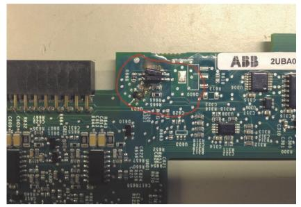
Figure 14: U605 burnt on control board
