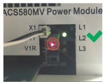
Figure 20: Fiber optic is ok
