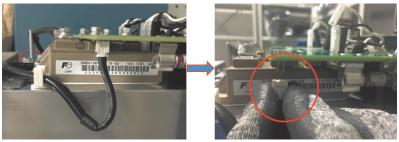
Step 5. Separate HCB board and CB board from holder.
