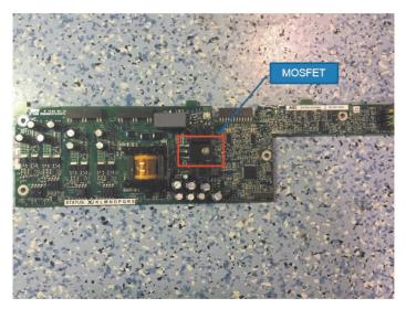
Use multimeter plus measure the resistance between source (test point 1 showed in under photo) and gate (test point 2 showed in under photo) of MOSFET, the resistance should be around 10Kohm.
