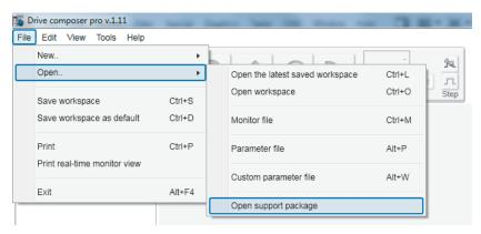
Figure: Opening the support package file in Drive composer
