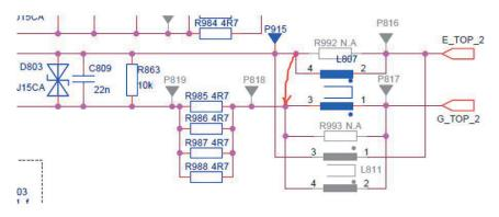
There are two group of coils inside of choke, one group connect with pin1 and pin3, another group connect with pin2 and pin4. Normally, pin1&pin2, pin3&pin4 should be open. Pin1&pin3, pin2&pin4 should be conductive.
