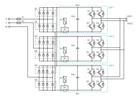
Figure 9: R9 power module main circuit diagram
