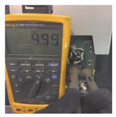
If the choke short inside, the measurement value will far less than 10Kohm. The following table showed the test point and allowed values:
