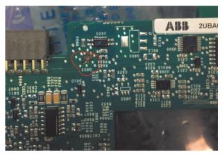
Figure 15: Q603 burnt on control board
