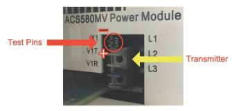
If there is no red light after connecting the pins correctly to the USB cable, the fiber optic sender is damaged.
