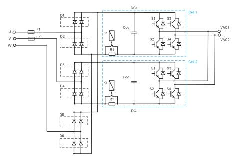
Figure 7: R7 power module main circuit diagram
