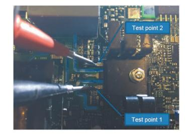
MOSFET failure happens when the resistance is almost 0ohm.
