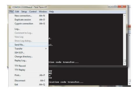
Select the PEBB1\_CellController.bin file from the MHDRE loading package (folder \02\_PowerModule SW).
