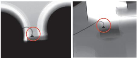
Figure 16: Delamination of fiber optic under X-ray
