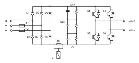
Figure 10: Main Circuit of Power Module
