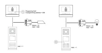
1. 1 level cascading connection for 2 outdoor stations with outdoor distributor
