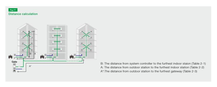
B: Max. distance from system controller to the furthest indoor station, calculation is based on total power unit of internal bus(check Table1) Table 2-1: Distance calculation for different cables (distance B)
