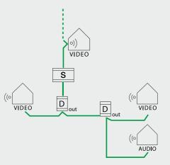
2 level cascading connection for 4 outdoor stations with outdoor distributor
