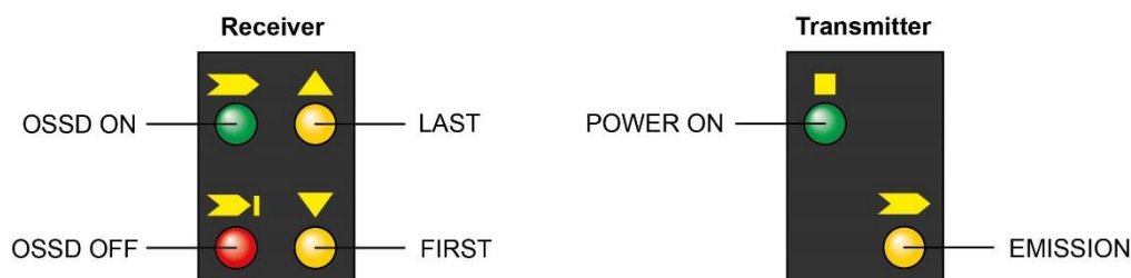
Figure 40 – LED display on the receiver and the transmitter
