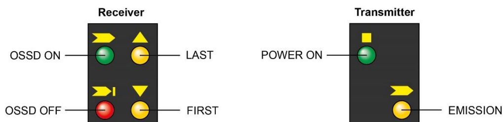
Figure 17 – Displays on transmitter and receiver
