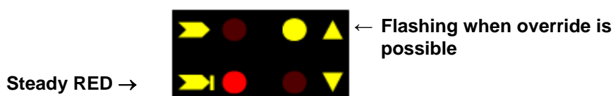
Figure 37 – Indication that the override function can be activated
