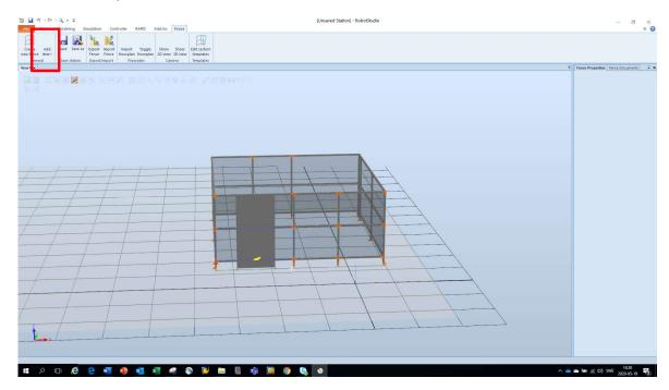
Click on left mouse button once and the door will be generated at the selected position. This can take a few seconds as RobotStudio will regenerate the fence.
