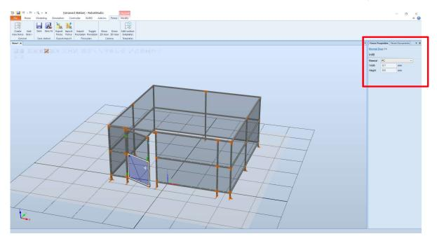
An overview of the current door settings will appear. It is now possible to change the dimensions, hinge side and hinge direction. Maximum door width is 1200mm.
