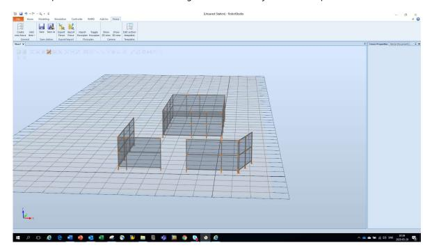
Be aware that the generated assembly drawings can be difficult to read and understand. The different fence sections will be printed in the same view and there is a risk that the fence sections in front and behind are mixed up.
