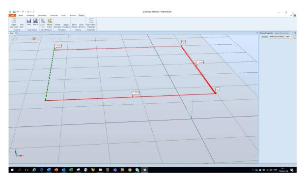
A realistic view of the fence will be generated when the double-click has been made. The creation of the fence can take a few seconds, depending on the size of the fence.
