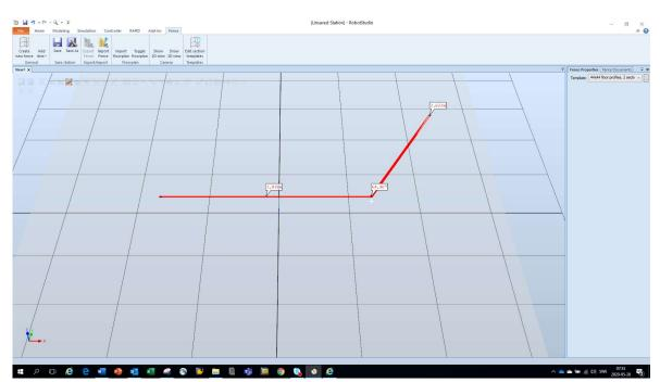
Click once on the left mouse button to create the angled fence section. Double click on left mouse button to finish the fence. Hinge brackets will be automatically added between all angled sections.
