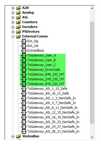
The blocks "...User\_A/B/C" are used to send memories, registers and/or inputs that are not **global** (see 1.5) variables. Please note that **exported** variables must be sent to a gateway by using these blocks.
