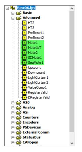
The two blocks "LightCurtain1" and "LightCurtain2" are blocks used mainly in press applications, combined with a light guard device and other sensors.
