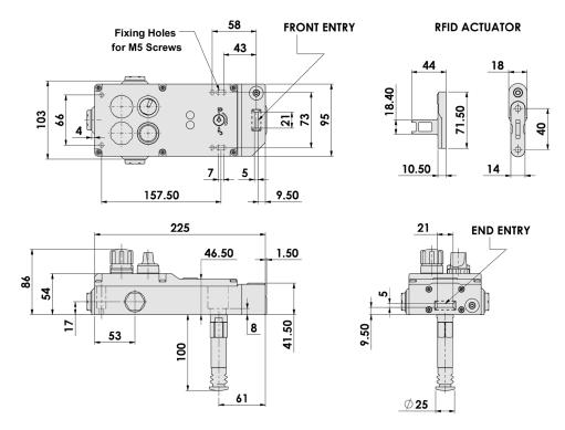
Dimensions - FHS GKey4 with rear handle and spring loaded catch
