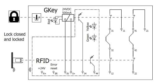
Actuator must be in place and RFID coding verified for the safety contacts to close.
