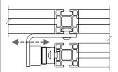
Note! To prevent damages on Magne, a separate door stop must be used.
