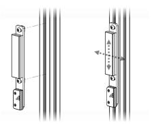
Note! Before tightening the screws, make sure the surfaces of Magne electromagnet and anchor plate are completely parallel, i.e. that full contact is obtained when the door is closed.
