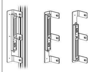
**Note!** If Magne M12-contact (cable) should be pointing up, use lower and center M6-installation holes.
