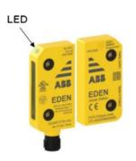
The LED currently fast flashes green if a valid Eva is within 2 mm from maximum detection distance. This is a non-safe indication that the mounting distance is on the limit and should be adjusted.
