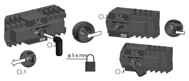
Figure 7 Locking the electrical operation
