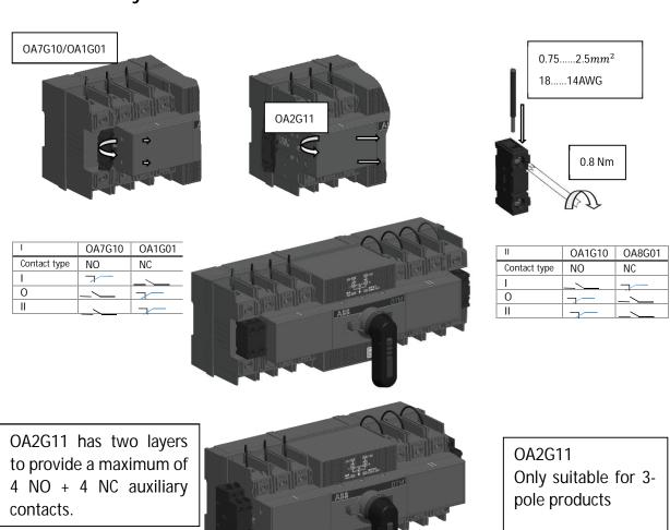
Figure 19 Auxiliary contact blocks
