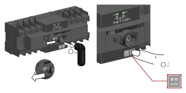
Figure 5 Selecting the automatic transfer OTM\_C\_20D switch to Auto mode
