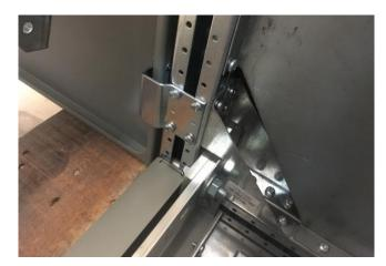
Place the Link to join with the next section
