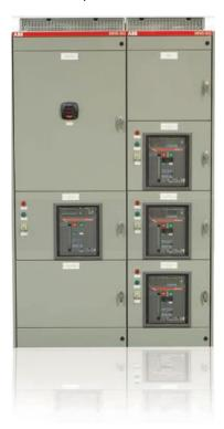
A continuous horizontal bus, rated 1,600 to 5,000 amps, distributes incoming power to all switchgear sections. The horizontal bus is located in the bottom half of each section, and for tie applications a similar assembly is used at the top of the section. Each section may contain a system of vertical bus, rated 1,600A up to 5,000A. The vertical bus is located in the busbar compartment, segregated from the device compartment.
