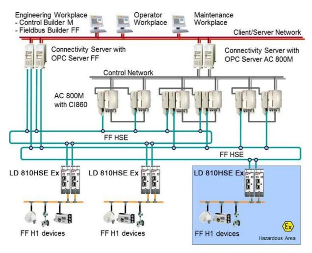
Sample System Structure with FF Network
