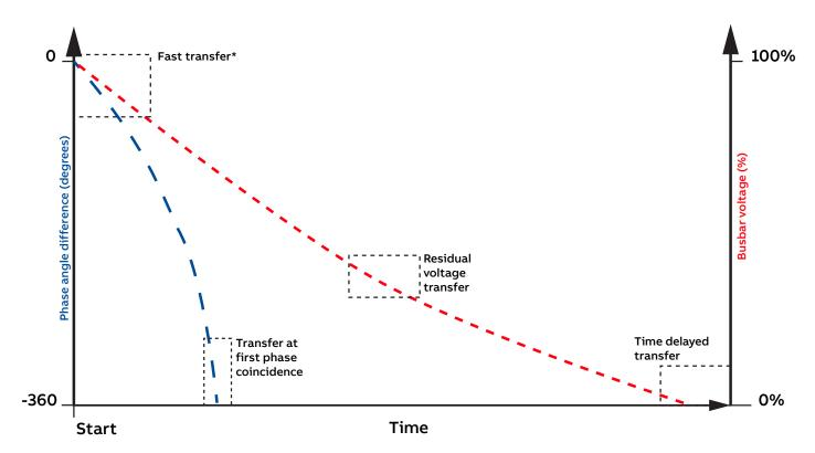
\*) The fast transfer mode offers two circuit breaker control schemes, simultaneous and sequential (break-before-make)
