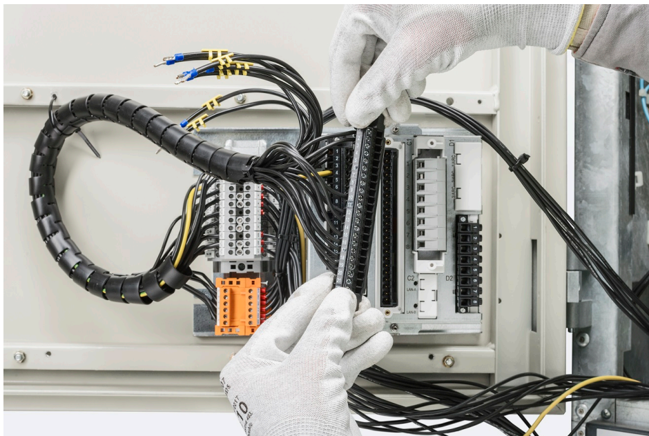
Figure 21: Connecting the pre-wired terminals to REX610
