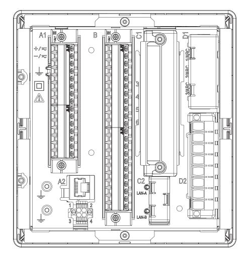
Figure 1. Hardware module slot overview of the REX610 relay
