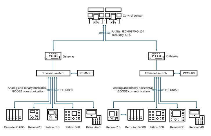
Figure 6. Communication example using Relion relays
