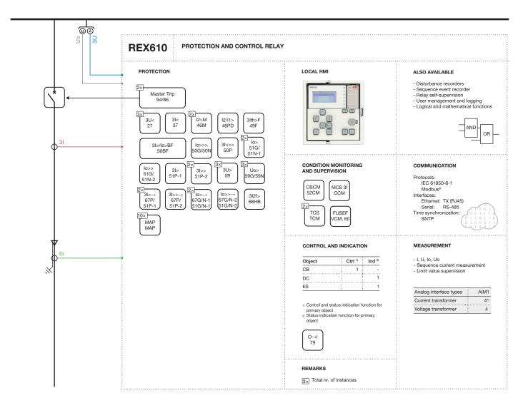
Figure 3. REX610 with CT and VT modules installed
