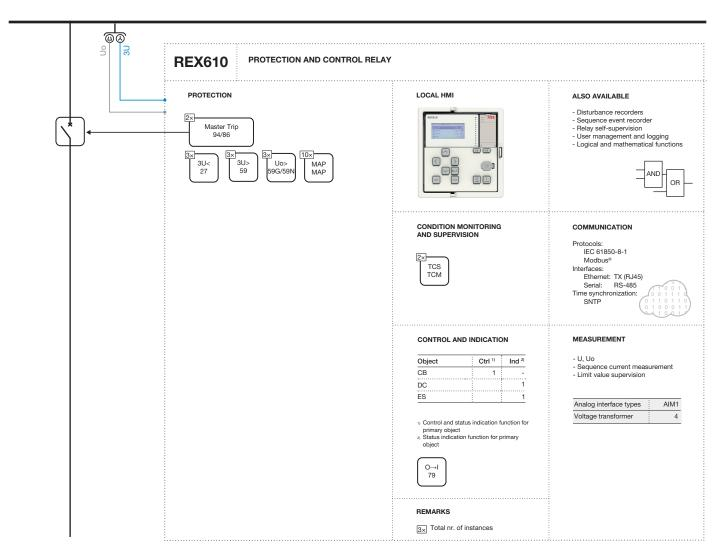
Figure 4. REX610 with VT module installed
