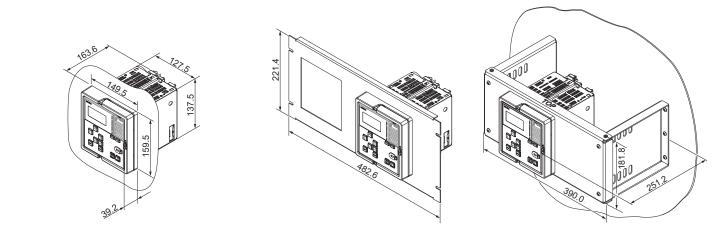
Figure 8. Flush mounting
