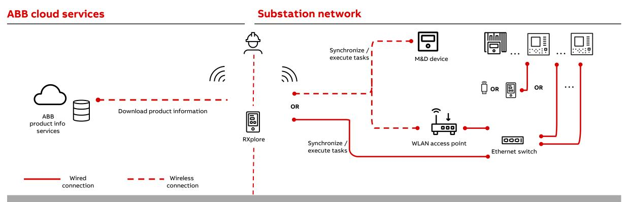
The app is connected either to the station network or to the ABB cloud services, but never at the same time
