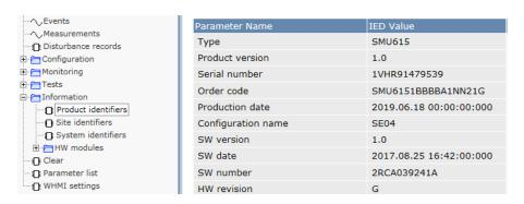
Fig. 2 Current firmware revision of the SMU615 Substation merging unit
