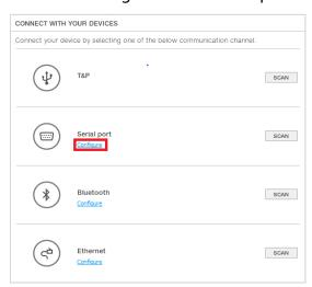
Select port name, baud rate (default: 19200), parity (default: Even), slave addresses (default: 1) of all devices connected via Modbus RTU to be updated.
