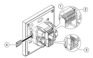
Fig. 4: Device overview of display rear side
