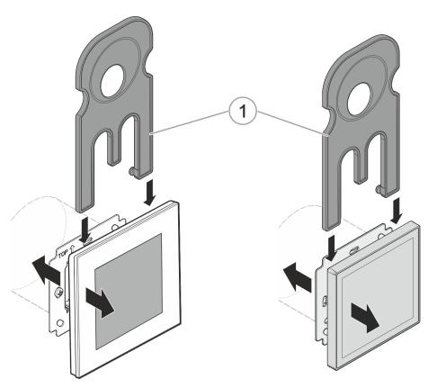
Fig. 15: Dismantling with removal tool
