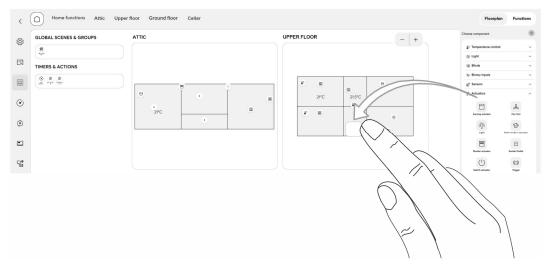
Fig. 17: Pulling the device out of the menu bar (example illustration)
