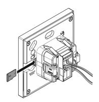
Fig. 34: Inserting the micro SD card (SDHC)
