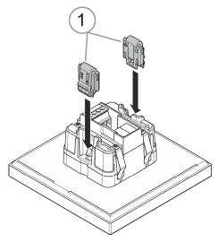
Fig. 13: Installation of the removal protection
