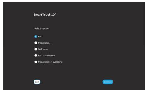
Fig. 18: Selection of system during initial commissioning
