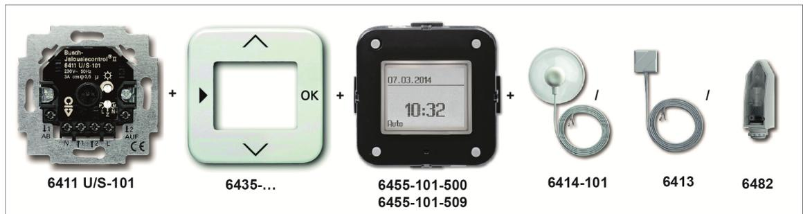
Only one brightness sensor 6414-101 or 6482 (for mounting outdoors) can be connected to the flush-mounted insert 6411 U/S-101. Also the simultaneous connection of a 6413 burglar alert sensor is possible.
