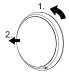
Twist the diffusor to the left and demount it carefully.
