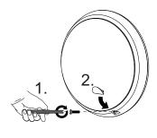
Secure the device with the special screw against vandalism.
