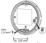
Insert the connecting cable through one of the
