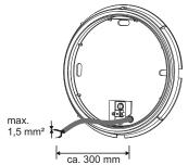
Insert the connecting cable through one of the
