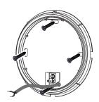
Fix the device base with suitable screws to the wall or ceiling.
