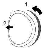
Twist the diffusor to the left and demount it carefully.
