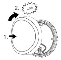
Connect the cable to the terminals at the backside of the diffusor.
