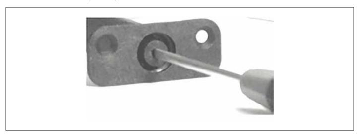
Using a corner of the screwdriver, "push in" an appropriate hole on the front side of the bolt (here, the wall thickness of the bolt is approx. 1 mm). After removing the screw cap, the spindle can be turned in an anti-clockwise direction using the screwdriver. This unscrews the bolt.
