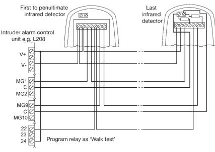
The terminating resistor (2.7 k ohm) must be looped into the last detector of a zone or sabotage zone. For a simpler installation, two free terminals are located on the housing of the detector.
