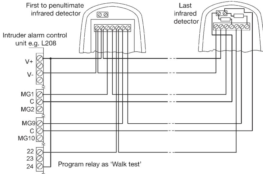
The terminating resistor (2.7 k ohm) must be looped into the last detector of a zone or sabotage zone. For a simpler installation, two free terminals are located on the housing of the detector.
