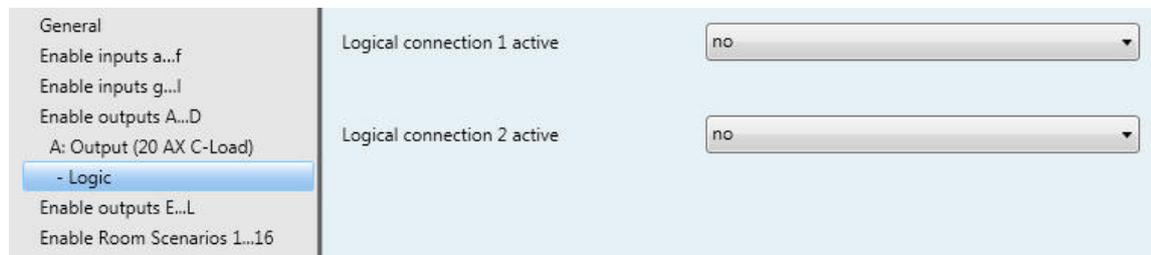
The function *Function Logic* provides up to two logic objects for each output, which can be logically linked with the communication object *Switch*.
