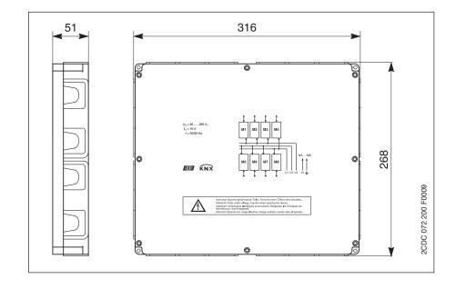
The device has eight module slots which are numbered as M1 to M8 respectively and when inserted, the module is connected to the mains supply voltage provided that the module requires the voltage for operation.
