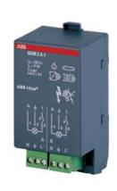
The 2-fold Switch Actuator Module can be operated in any module slot of the Room Controller Basis Device. It switches two independent groups of electrical loads such as fluorescent lamps using relay contacts. The outputs are distinguished by a high switching current. Both the incoming supply and the internal voltage are supplied via the Room Controller Basis Device. Contact is automatically established when the modules are snapped in place.
