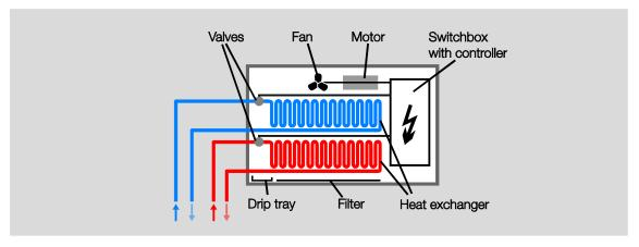
The fan blows air past the heat exchanger and into the room through a filter. The air is heated or cooled in the heat exchangers and thus generates the desired room temperature. The fan is driven by a motor. The motor and the valves are controlled by a Room Master.
