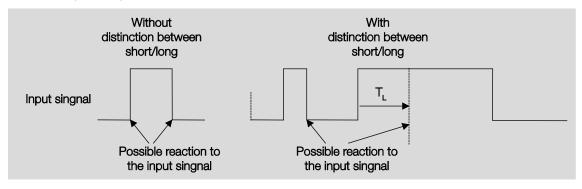
$T_{\text{L}}$  is the time duration from where a long operation is detected.
