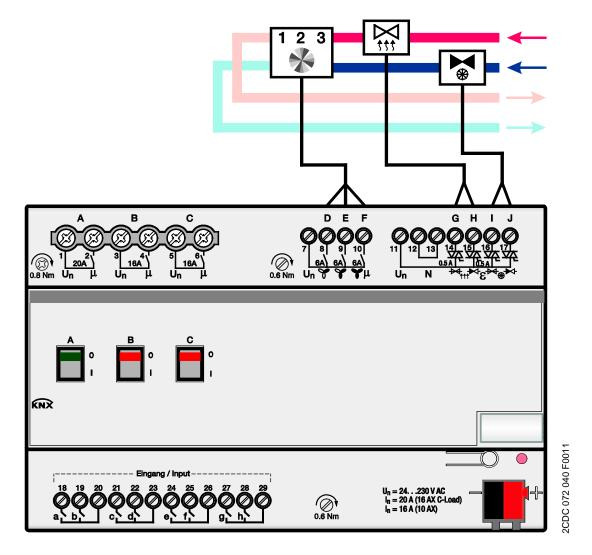
Even the offset of the set point value as well as changeover of the operating modes is implemented by the thermostat. The sensors can be connected directly to the Room Master in order to consider the monitoring of the condensed water and the window contact.
