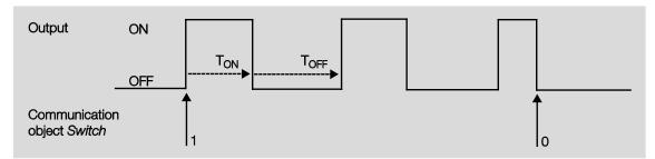
The switch on time  $(T_{ON})$  and switch off time  $(T_{OFF})$  during flashing can be programmed.
