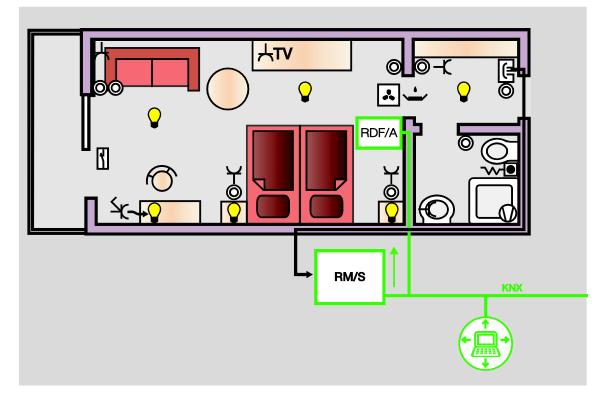
All lights are switched off directly via the outputs with delayed event 2, after the delay time has timed out. Various binary inputs are blocked. The thermostat, e.g. RDF/A receives a telegram via the bus to change to mode *Building Protection*.
