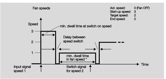
\* The parameter *Minimum dwell period in fan speed in s [0...65,535]* in the parameter window *Automatic operation* is only active and programmable, if the option yes has been selected in the *Enable automatic operation* parameter. In the parameter window *Fan*, you can find the parameter *Enable automatic operation*.
