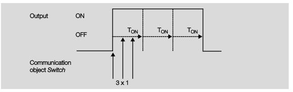
If the device receives a further ON telegram when the staircase lighting is switched on, the staircase lighting time is added to the remaining period.
