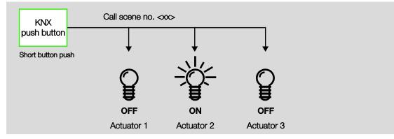
A scene number is sent with the telegram value which must correspond with the scene number in the parameters of the Room Master.
