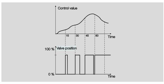
With pulse width modulation, a relatively accurate control of the temperature can be achieved without any resulting overshoots. Simple, attractively-priced control valves can be used. The positioning frequency of the control valve is relatively high.
