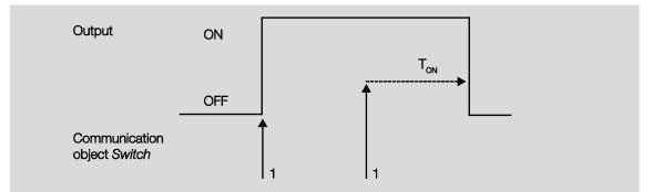
The response is the fundamental response of the staircase lighting function.
