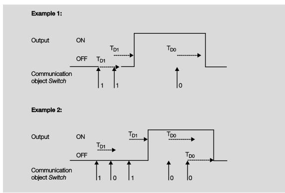
The delay time  $T_{D1}$  or  $T_{D0}$  starts after a switch telegram, and after it has timed out, the output executes the switch telegram.
