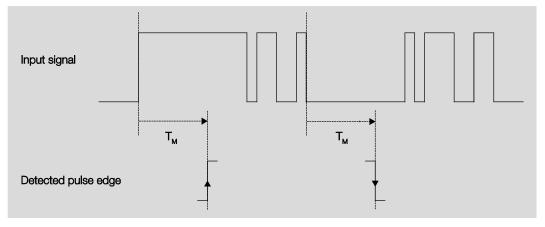
In only two cases, no further edge changes occur within the minimum signal duration  $T_M$  after a change of edge. For this reason, only both of these are detected as valid.
