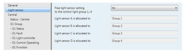
If several light sensors are assigned to an output, it is necessary to define which sensor value is used as the actual value (input variable) for the control circuit.
