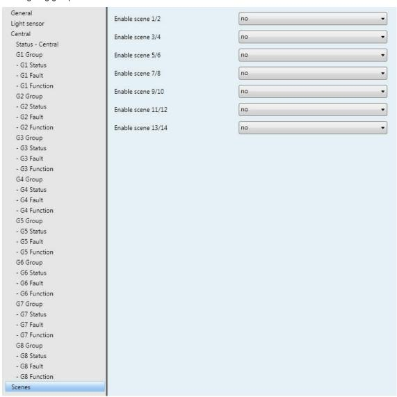
In order to parameterize a scene in the ETS, the corresponding parameter window Scene x/y (x/y = 1/2, 3/4, 5/6...13/14) must be enabled.
