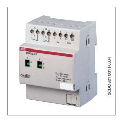
The 2-fold DALI switch actuator is a DIN rail mounted device for insertion in the distribution board on a DIN rail in accordance with DIN EN 60715. Using floating contacts (normally open contacts), the DALI switch actuator switches 2 independent electrical loads through a switch contact each.
