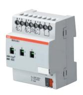
The Energy Actuator is a modular installation device in Pro *M* design for installation in the distribution board. The device is especially suitable for switching loads with high peak inrush currents such as lighting equipment with compensation capacitors or fluorescent lamp loads (AX) to EN 60 669.
