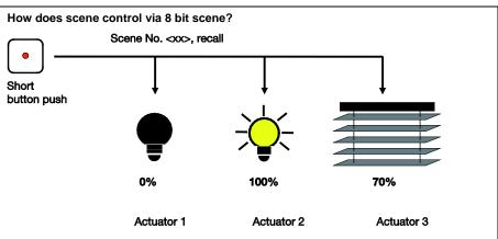
Fig. 3: Recalling and storing via "8 bit scene"
