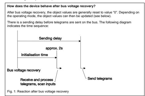
The inputs are scanned after the initialisation period and the object values are updated if the parameterization has been set accordingly. If the input is actuated at bus voltage recovery, the device will behave as if the actuation commenced at the end of the initialisation time.
