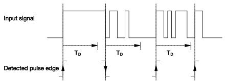
After detection of an edge on the input, further edges are ignored for the debounce time  $T_D$ .
