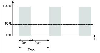
During  $t_{ON}$ , the valve is triggered with OPEN ("ON phase"). During  $t_{OFF}$  the valve is triggered with CLOSE ("OFF phase"). If  $t_{ON} = 0.4 \times T_{CYC}$ , the valve is set at approx. 40%.  $T_{CYC}$  is the so-called PWM cycle time for continuous control.
