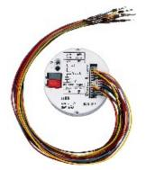
The device has 12 channels, which can be parameterized individually in the ETS, as inputs or outputs.
