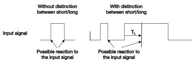
Fig. 2: Distinction between short/long operation for "Switch sensor" mode
