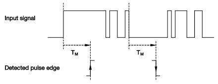
As only two edges remain stable for the minimum signal time  $\mathsf{T}_{\mathsf{M}},$  only these are detected as valid.
