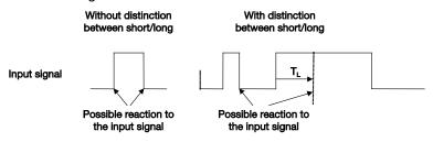
Fig. 3: Distinction between short/long operation for function "Switch"
