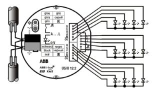
Series resistors for operation of the LEDs are integrated into the device. The maximum output current is 2 mA per LED.
