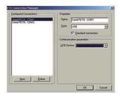
With the USB Interface USB/S 1.1, you are properly connected to the ABB i-bus®. It enables communication between the ETS 3 and the ABB i-bus® system that is for programmed. The communication between the two bus systems is indicated by the EIB-LED and the USB-LED. The USB/S 1.1 functions with the new ETS3 program onwards. The USB Interface is simply connected to the ABB i-bus® and then to the USB. The USB/S 1.1 is automatically detected under the pc operating system and installed.
