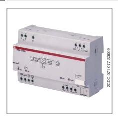
The Uninterruptible Power Supply Unit NTU/S 12.2000.1 is a modular installation device in ProM-Design, for snapon mounting on a 35 mm mounting rail in a universal, wall-mounted or ceiling panel distribution board as well as in distributed surface mounted housings. The power supply delivers sufficient power for all types of demanding applications with a buffered output voltage of 12 V DC and a maximum output current of 2 A.
