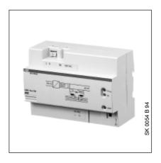
The power supply unit produces and monitors the power for the EIB system. The bus line is isolated from the power supply with the integrated choke.
