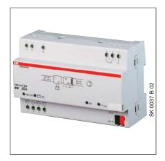
The Uninterruptible EIB / KNX Power Supply produces and monitors the EIB / KNX system voltage. The bus line is decoupled from the power supply with the integrated choke.
