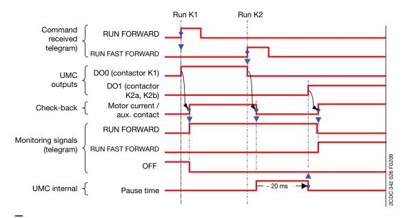
Timing Diagram for Pole-Changing Starter
