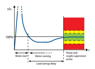
The load startup delay time allows to delay the low-power protection functions at startup. This can be used for example to allow a pump to built up pressure before the low power protection becomes active
