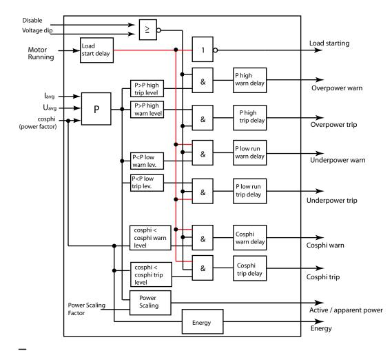
The following block diagram shows the data flow of the power supervision in the UMC/VI15x and the generated signals.
