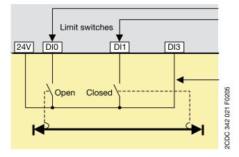
DI0: Motor off, start only in Closed direction DI1: Motor off, start only in Open direction DI3: Fault: motor stops
