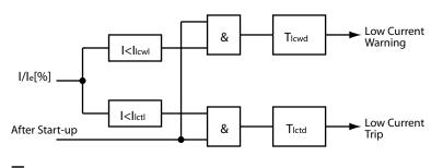
Signal flow of the low current protection function.
