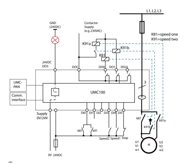
Circuit diagram of the UMC for controlling dahlander motors. The checkback contacts k81/k91 are optional
