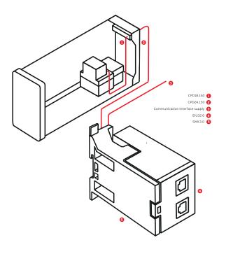
Communication adapter and accessories in a draw-out installation. The fieldbus node is outside the drawer so no drops are required. To keep the communication interfaces powered in case the drawers are withdrawn they must be powered separately (not shown here).
