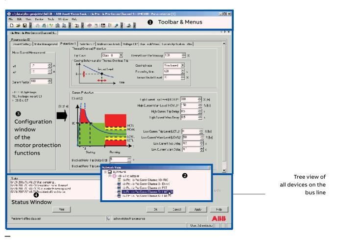
UMC100.3 configuration tool Asset Vision Basic with the motor protection configuration window 3. In 1 the toolbar of the tool is shown. 2 provides a network view with all the devices accessible on the PROFIBUS DP line. 3 contains a window to display messages and buttons to quit or adopt the parameter changes.
