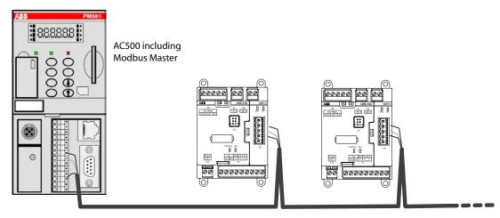
Modbus Line with MRP31 and UMC100.3. Use standard Modbus cable for wiring
