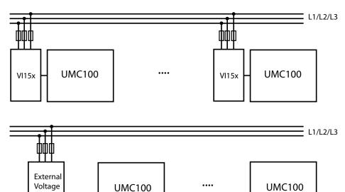
A low voltage situation can be detected either by the VI15x module or using an external voltage monitoring relay. In the latter case the low voltage signal has to be wired to all motor controllers
