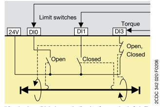
\*) Start is only possible in the opposite direction after resetting the fault. The torque signal has to disappear within 0.5 s otherwise a fault is generated again.
