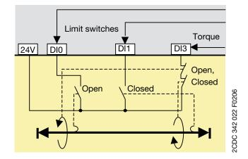
DI0: Preparation for Open limit motor off
