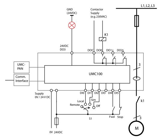
From the requirements you can see that the three control places Digital Inputs, Fieldbus and LCD are used. Furthermore start/stop commands from the different control places shall be blocked or released depending on the Fieldbus and S1 status. Therefore the different modes can be used.
