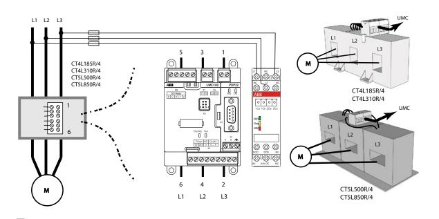
Wiring scheme when using ABB CT4L/5L current transformers
