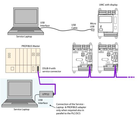
Connection of a service laptop using a USB cable connected with the UMC100 LCD panel (point-to-point) or UTP22-FBP (for a whole PROFIBUS line)
