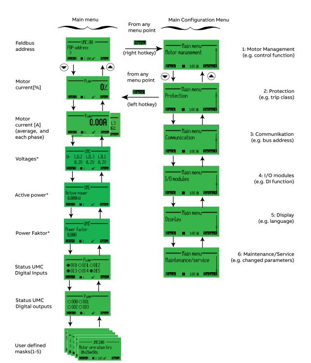
With the right soft key **section** you can enter the selected submenus which are described in the following sections. The masks shown with a star \* are only displayed if the voltage module is present.
