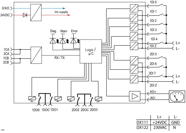
Wiring diagram of the DX1xx modules
