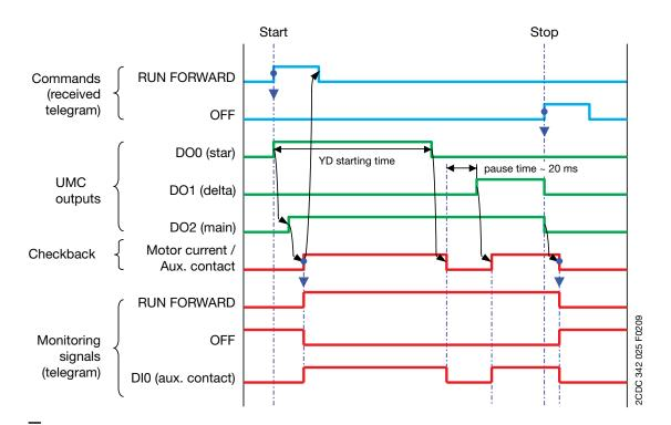
Timing Diagram for Star-Delta Starter
