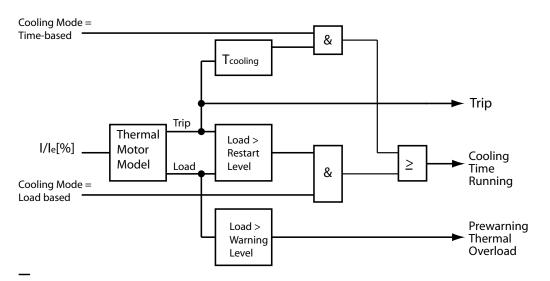
Signal flow of the thermal overload protection
