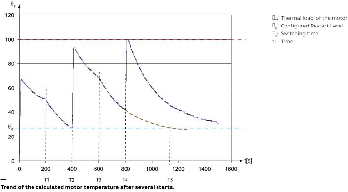
The motor trips after the third start because the motor was started too frequently in the given time
