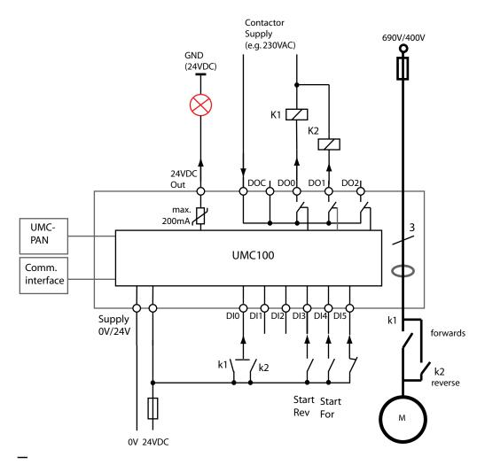
Circuit diagram of the UMC for controlling a motor in two directions of rotation. The checkback contacts k1/k2 are optional
