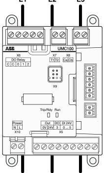
If the phase sequence supervision is active the phases must be fed through the UMC in the shown order
