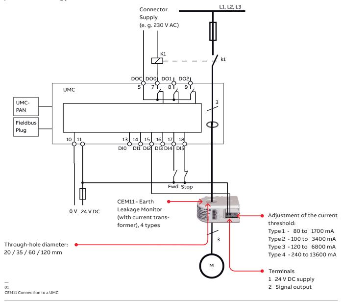
By nature, earth fault sensors encounter all kind of disturbances inserted through the motor feeding lines. Therefore the evaluating unit should foresee some kind of filtering to suppress erroneous activations of the output due to disturbances.
