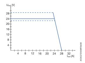
Characteristic curve of output at  $T_{\rm a}$  = 25 °C
