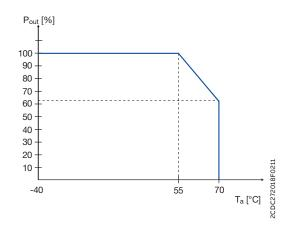
Characteristic curve of temperature at rated load
